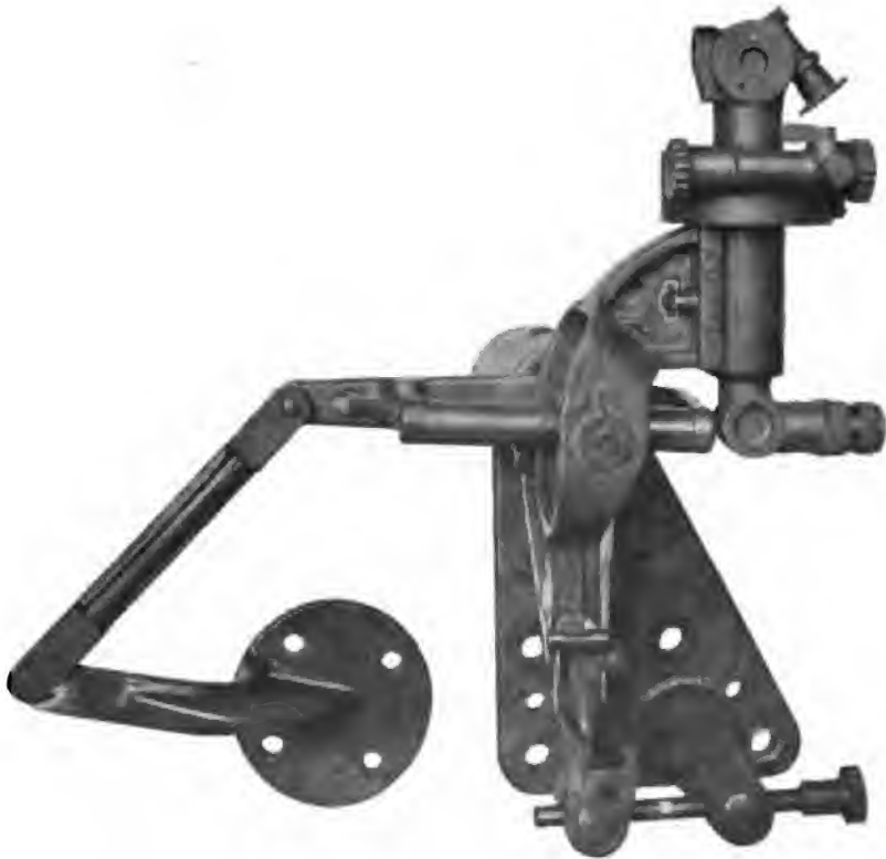
PANORAMIC SIGHT MOUNTED ON AUTOMATIC SLOPE COMPENSATING MECHANISM.
